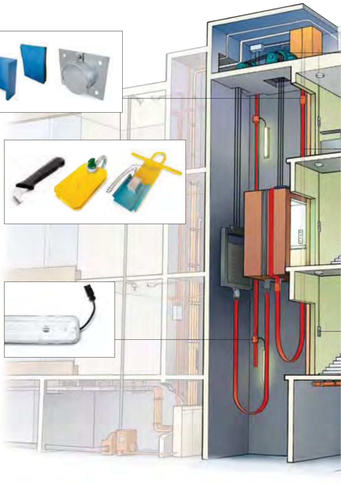
Installation tools for simple installation of FL, FM and FH cables
